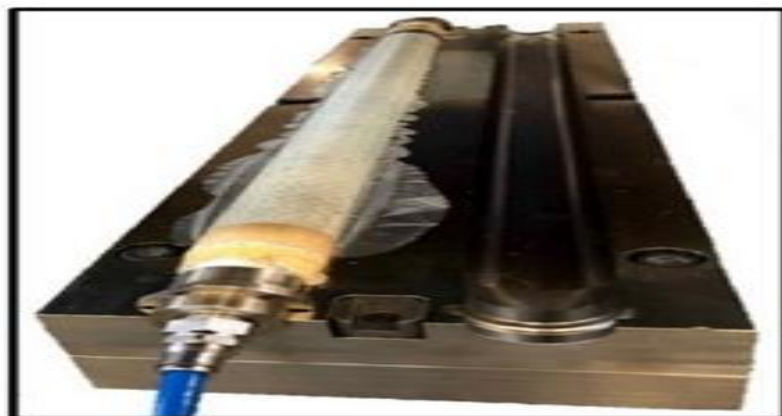
Image 7. Glass/PA 6-based composite beam material sample with 3D braiding structure, 2019
