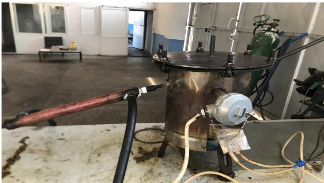
Figure 2. Pyrolysis setup for fuel production
